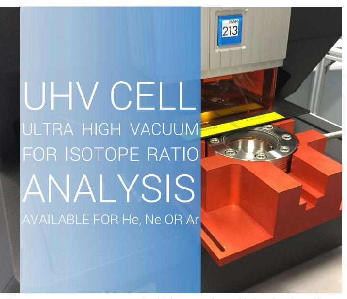
Ultra high vacuum laser ablation chamber with flush window and bolts for safe operation
